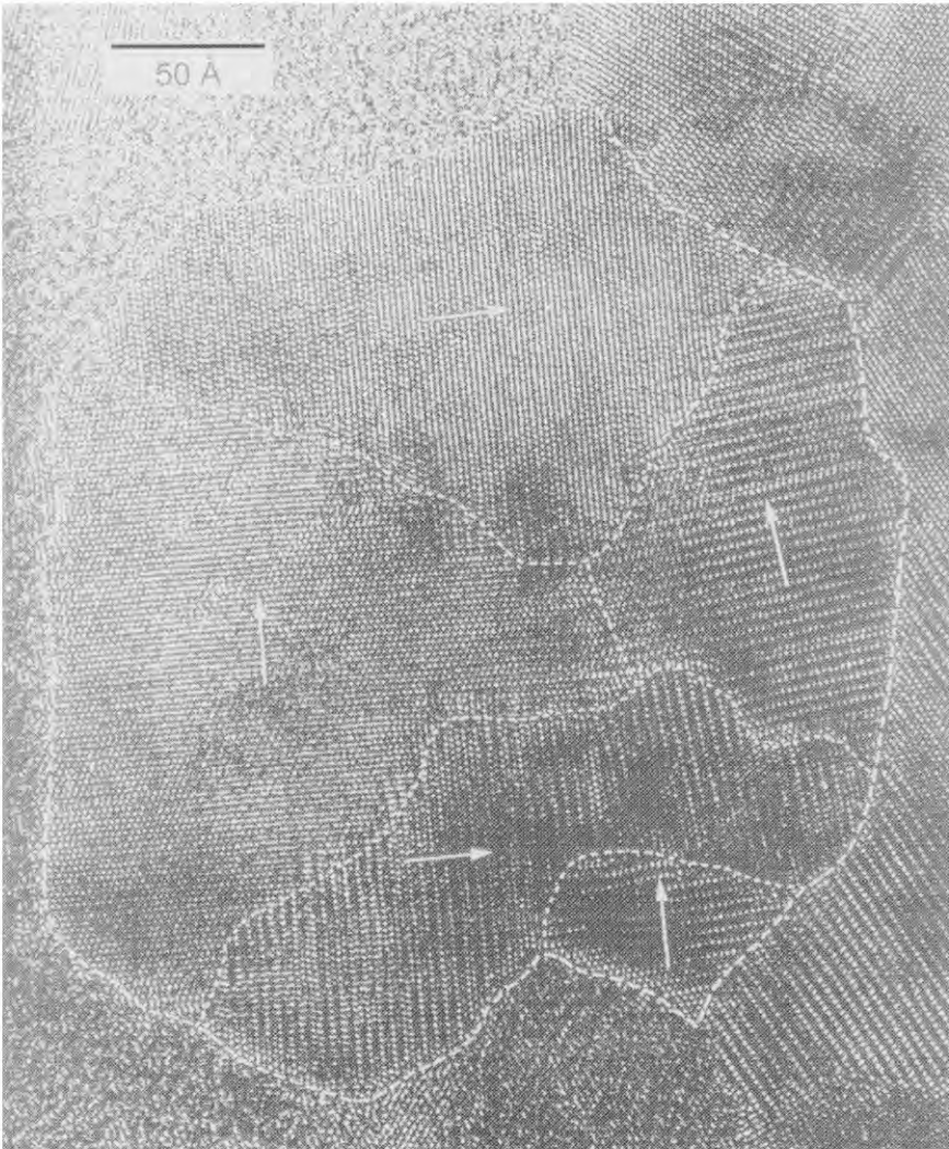
Fig. 5.12. TEM image of a bicrystal of \text{Co}_{75}\text{Pt}_{12}\text{Cr}_{13} on an underlayer of \text{Cr} ( \text{V}_{20} ) (Peng et al. 1995).
